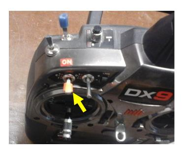
We do use fuel tubing on our gyro and mixing switches, one on each side of the transmitter (you can see the blue-tubing clad gyro switch at the back of the transmitter). We also use the nice Spektrum lady's voice to let us know when a switch is thrown, although she can be quickly drowned out by loud music, voices or engine noises (another reason not to carry on loud conversations when flying – you may be keeping your fellow fliers from hearing their radios).
