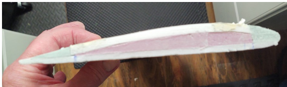
(Left) Wing at tip, showing LE and TE shaping.
