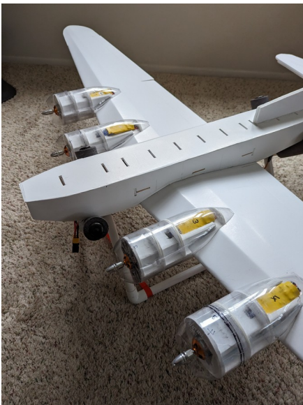
(Left) Soda bottle nacelles are hard to see, but they're there. Note fuselage crutch, slotted for bulkhead tops.
