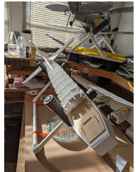
(Left) Soda bottle nacelles are hard to see, but they're there. Note fuselage crutch, slotted for bulkhead tops.
