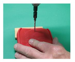
Step 1 (*left*): Using a soft plastic lid (yes, I like raisins in my breakfast oatmeal!), drill a series holes slightly smaller in diameter than your machine screws' thickness.
